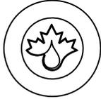
**Single Test Cycle** - place magnet on maple leaf logo. When bottom horizontal bar lights up, remove magnet to initiate single cycle. Pump will run for programmed period of "On Time".
