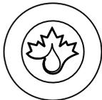
**"Off" Time Programming** - place magnet on maple leaf logo. Remove when top 4 bars light up. You can now program "OFF" times. Quickly replace and remove magnet till chosen parameter is shown - 1 through 5.
