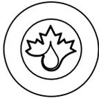
**Continuous Cycle** - place magnet on maple leaf logo. When bottom 2 horizontal bars light up, remove magnet to initiate continuous running of pump. Turn off power or put magnet back to stop pump.
